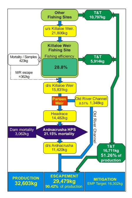
Figure 5-6: A summary of the NUIG analyses of silver eel production and escapement in the River Shannon during the 2016/17 eel migration season, based on one weir fishing efficiency value (28.8%), actual catch and normal calculation protocols.
