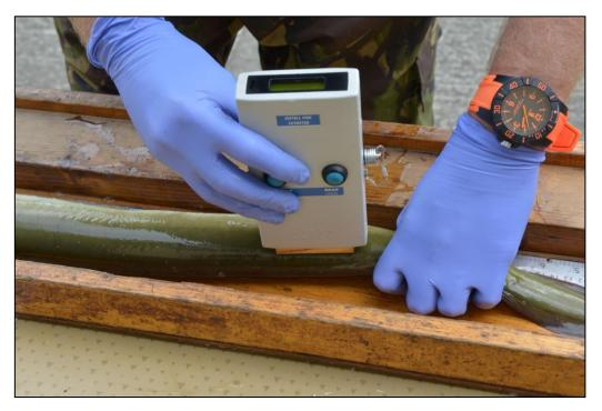
Figure 6-32: Using the Distell fish fat meter to measure % fat content in LLE yellow eel.
