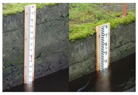
Figure 5-20: Depth gauge installed at silver eel weir on Clarebane River, 2015, pictured at 0.5 metres depth on November 6<sup>th</sup> (left) and 1.3 metres depth on November 20<sup>th</sup> (right), (Photos: R. Cruikshanks)
