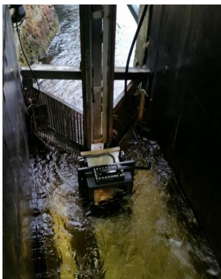
Fig 3.1. Erriff upstream trap with VAKI Riverwatcher counter and Biomark antenna (dark rectangular unit).
