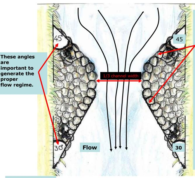
The largest heaviest stones available should be used at the outer tip of each deflector where the maximum erosive pressure will be generated by river flows.
