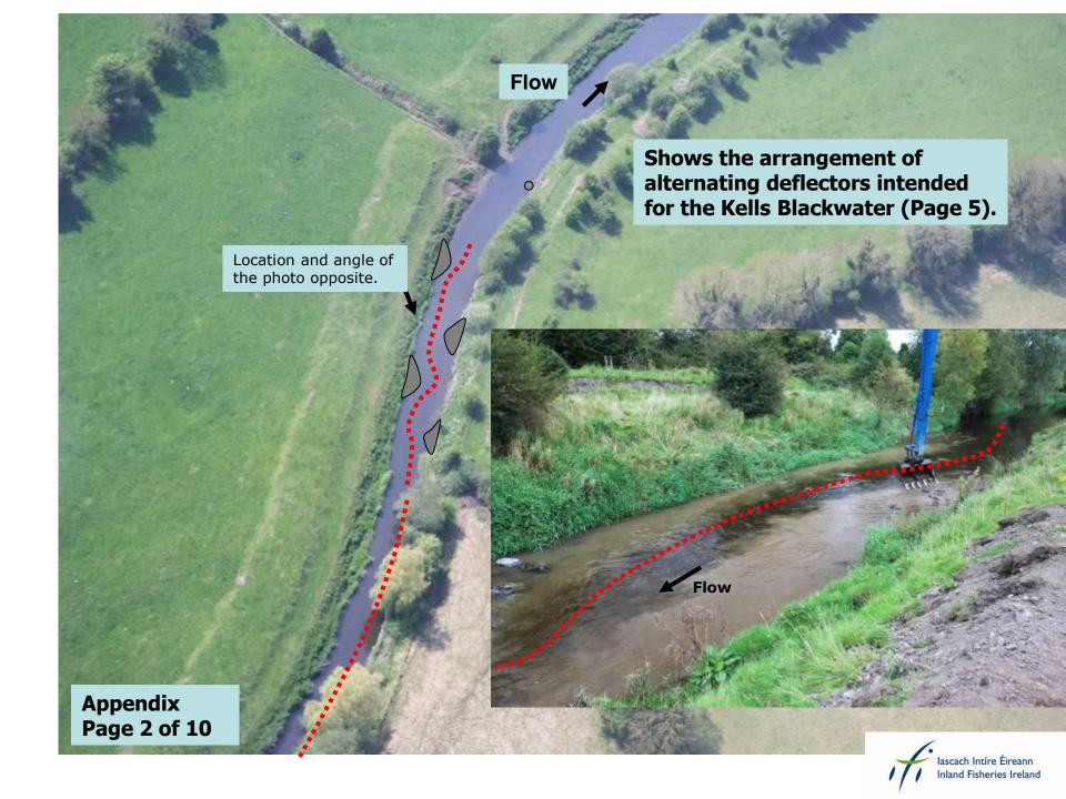
Another example of the ideal arrangement of deflectors for the reach of the Kells Blackwater. Note the placement of all boulders in the thalweg. See next page for an illustration of thalweg shape and size and boulder placement.
