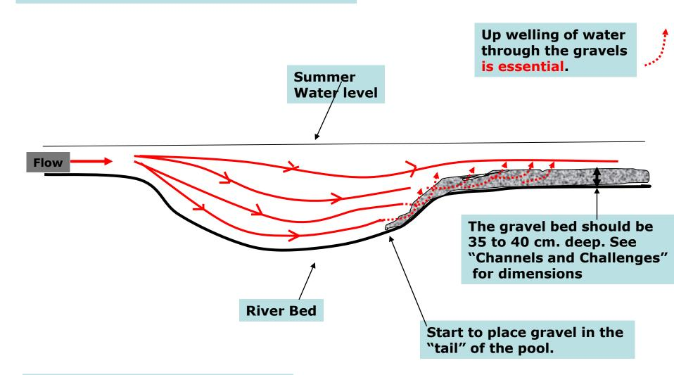
The pool and gravel bed should be about the same length – about 1.5 times the channel width.
