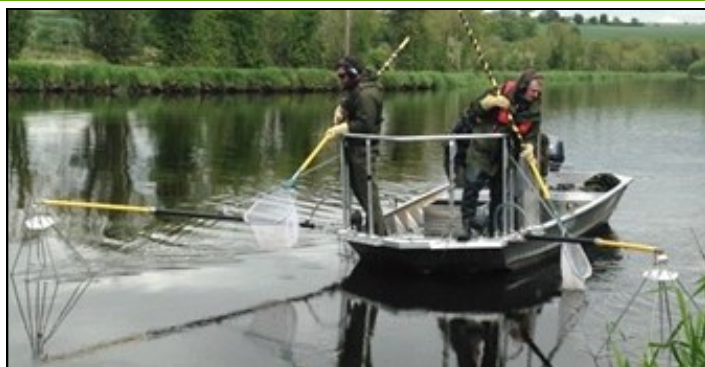
Boom-boat electrofishing on the Barrow
