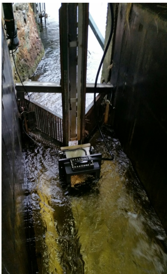
Fig 3.1. Erriff upstream trap inscale with VAKI Riverwatcher counter and Biomark antenna (dark rectangular unit).
