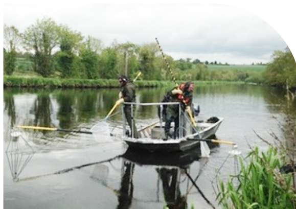
▲ Inland Fisheries Ireland staff using boom boat electrofishing equipment to assess fish populations
