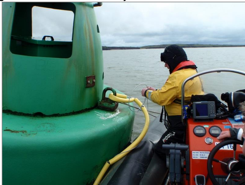
Plate 3.6. Attaching an acoustic receiver and tether to a Port of Waterford navigation marker buoy off Creadan Head.
