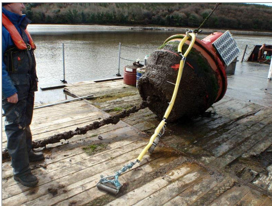
Plate 3.5. Attaching an acoustic receiver and tether to a Port of New Ross navigation marker buoy in the River Barrow at Fisherstown.
