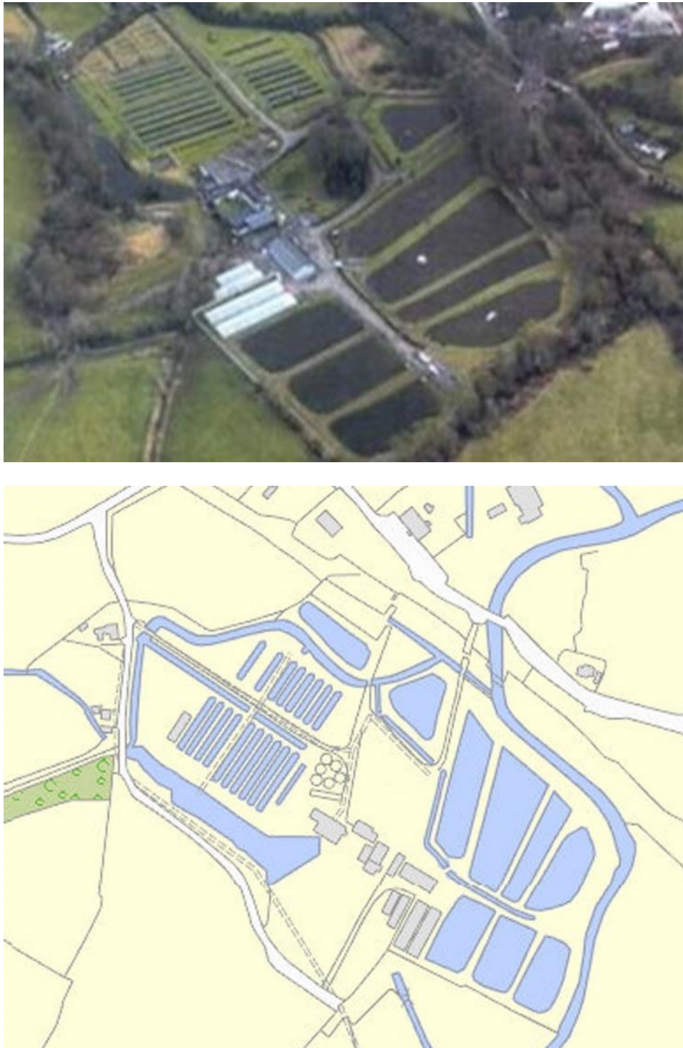
Figure 2: Aerial photo and schematic diagram showing the layout of buildings, raceways and ponds at the Roscrea Fish Hatchery.
