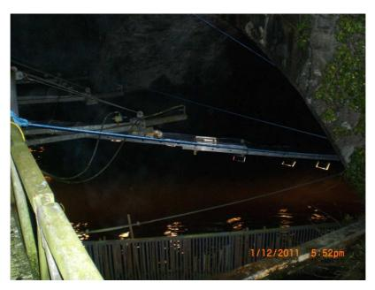
Figure 3.2: Experimental use of a light array and DIDSON™ camera at Killaloe for investigation of silver eel responses to light.
