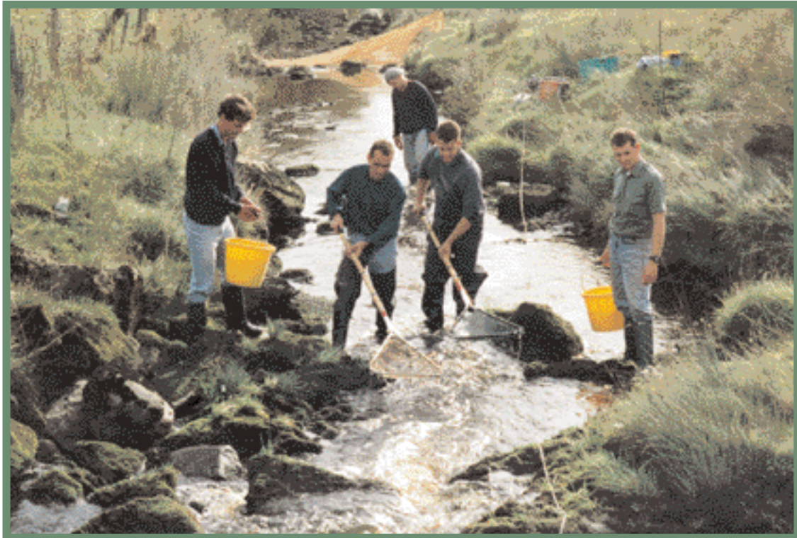
Electro-fishing survey in a headwater stream
