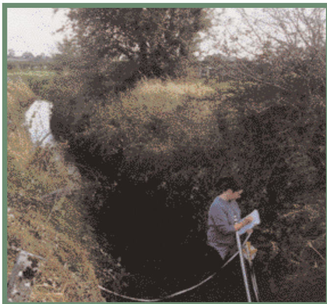
Recording channel width to estimate area
