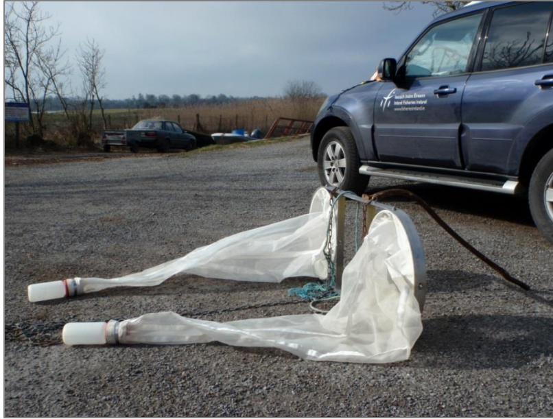
Plate 3.1. Bongo net used to undertake juvenile fish surveys.
