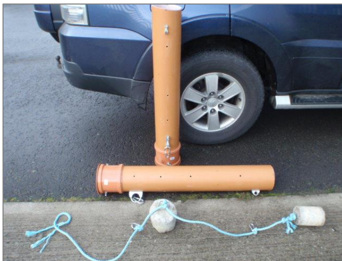
Plate 2.18. A pair of river lamprey traps prior to deployment
