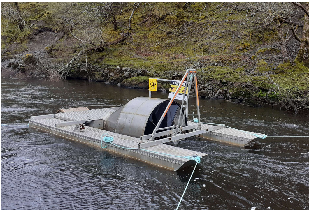
Plate 3 Rotary screw trap for capturing smolts in operation on the main river channel at Erriff Bridge. This trap was deployed during April-May in 2024 primarily for the purposes of capturing emigrating salmon and sea trout smolts for PIT and DST tagging (Section 4.2.3)
