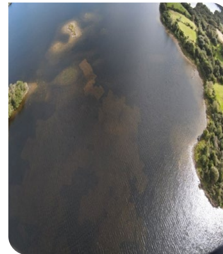
Image: Jute matting laid on the lake bottom visible from drone footage.
