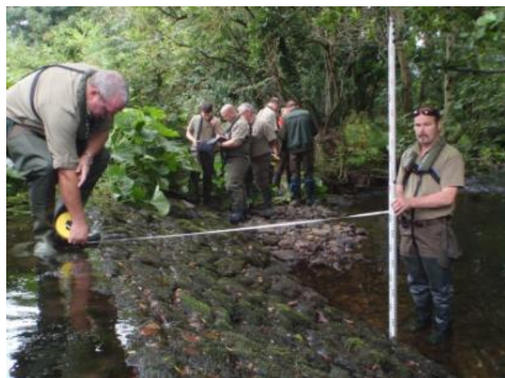
Figure 18 - Using tape and staff to record
