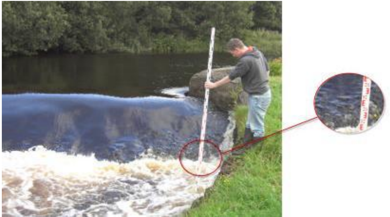
Figure 14 - Use of levelling staff for detailed measurements
