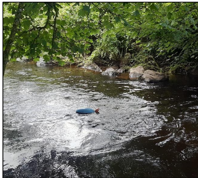
Plate 3: Multi-parameter IoT device floating in the Mount Nugent. Sensors include temperature, dissolved oxygen, pH, turbidity, and conductivity. Data transmits to an online dashboard in near real time, every 15 minutes.
