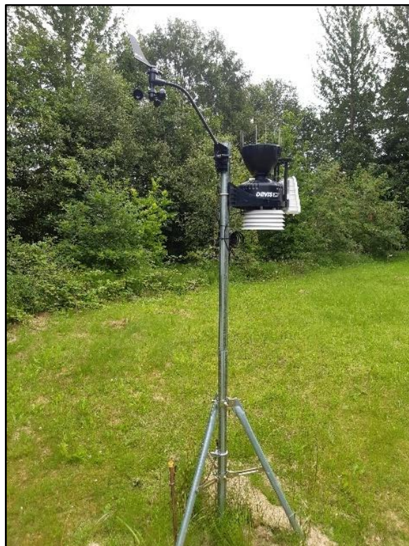
Plate 1: Weather station installed at Inland Fisheries Ireland Lough Sheelin base, transmitting meteorological data in near real-time.
