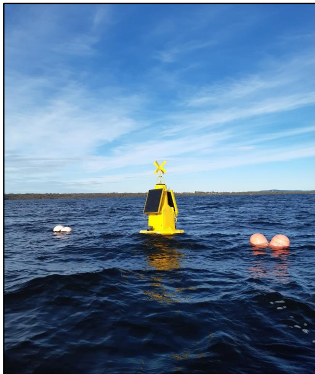
Plate 2: Data buoy platform installed on Lough Sheelin. Stored inside is a multi-depth thermistor chain surface to bottom (0.5, 2.5, 4.5, 6.5, 8.5, 10.5 and 12.5), and multi-parameter sonde at the surface (0.5m) recording temperature, dissolved oxygen, conductivity, and chlorophyll-a. Data transmits in near real time every 10 minutes to an online dashboard.
