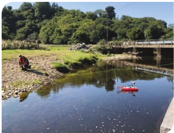
Image: Measuring flowing using an acoustic doppler current profiler (ADCP) on the Dinin River, Co. Kilkenny
