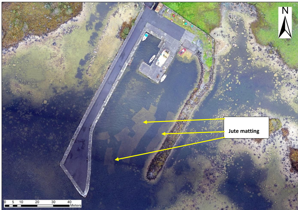
Fig. 2.10. UAV orthomosaic image showing jute matting in Kilbeg Pier, Lough Corrib, 7 th October 2020.
