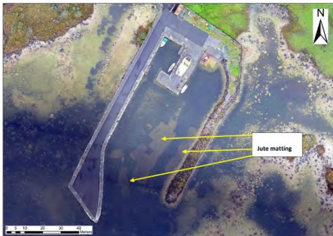
Fig. 7.1. Aerial imagery of Curley waterweed in L. Corrib and the management of extensive beds by covering with jute matting. This material decomposes into the lake bed having smothered the invasive weed, allowing natural vegetation to re-establish
