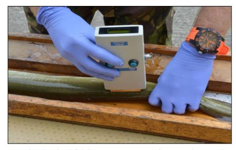
Plate 6-1 Using the Distell fish fat meter to measure % fat content in LLE yellow eel.
