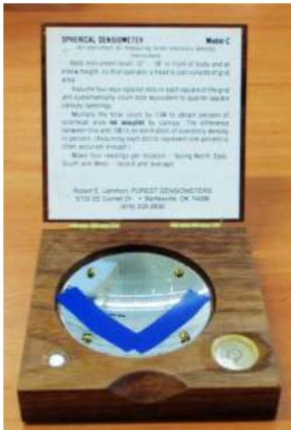
The densimeter consists of a curved concave reflecting mirror and has 37 grid intersection forming 24 squares. Only 17 of the line intersects are used as recording points by taping a right angle on the mirror surface as shown in Figure 4. Canopy density/closure is measured at 4 or 8 points in the stream depending on width.
