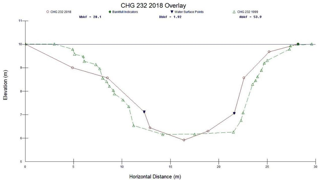
**Figure 3.6. Comparison of cross-sections from 1999 (pre-maintenance – green line) and 2018 (black line) for chainage 228 (top) and 232 (bottom). See photographs below.**
