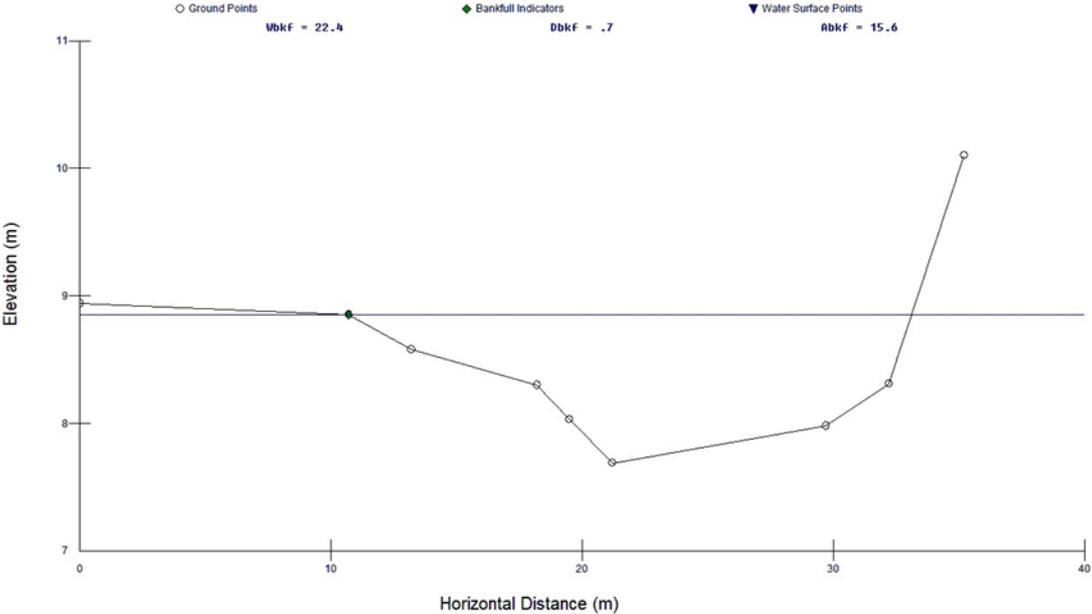
Figure 5.5. Channel dimensions at location of cross-section levelling.
