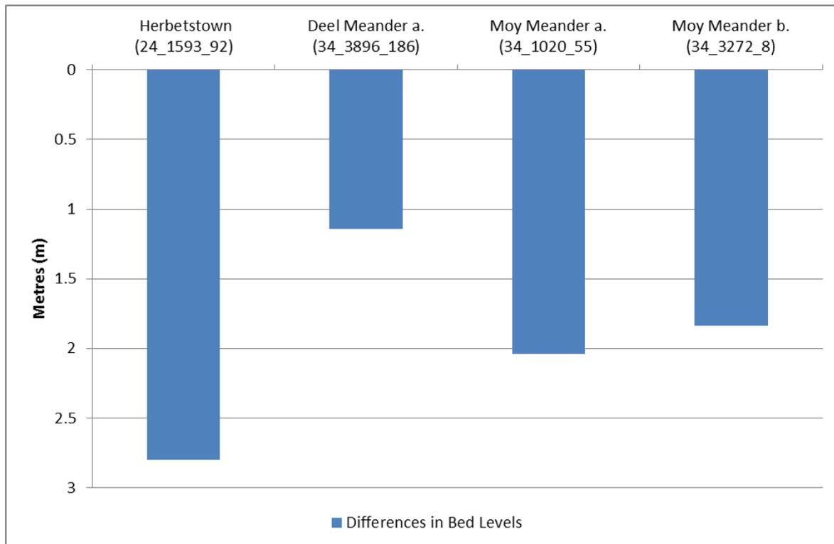
**Figure 5.8. Stage or vertical height (m) differences between existing river bed level adjacent to meanders and bed level in meander. 0 on x axis is the current bed levels of each meander.**
