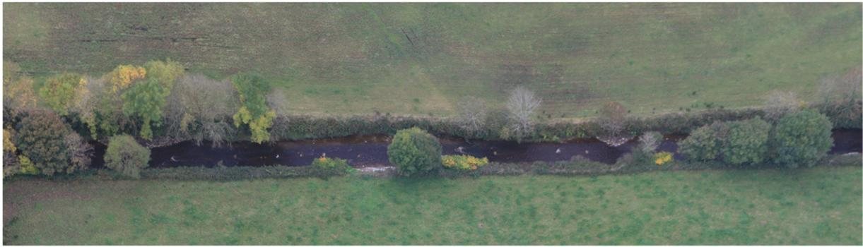
**Figure 4.8. Aerial view of the River Maine experimental post works October 2009 (note alternating deflectors and random boulders).**
