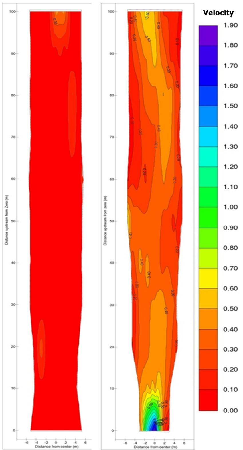
**Figure 4.14. Velocity (m/sec) contour plots of the 100m upstream of Milltown Bridge pre (left – 2013) and post (right – 2015) removal of horseshoe weir and construction of alternating deflectors.**
