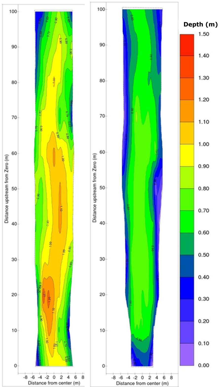
**Figure 4.13. Depth (m) contour plots of the 100m upstream of Milltown Bridge pre (left – 2013) and post (right – 2015) removal of horseshoe weir and construction of alternating deflectors.**
