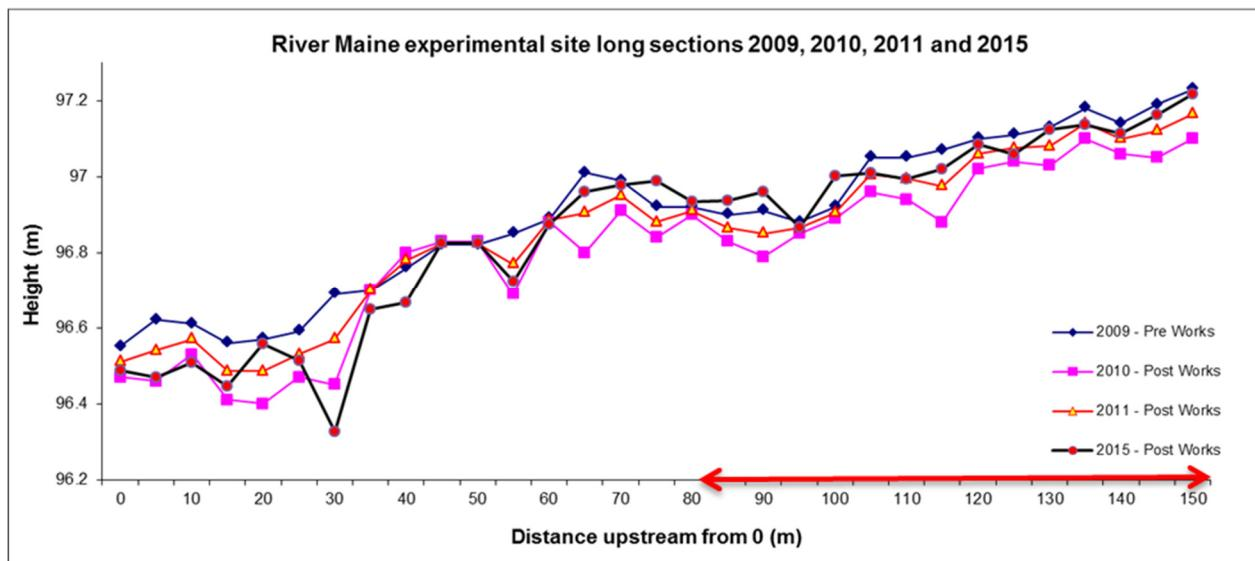
**Figure 4.10. River Maine experimental site long sections pre (2009) and post works in 2010, 2011, 2015 (arrow indicates location of depth contour plot in Figure 4.11).**
