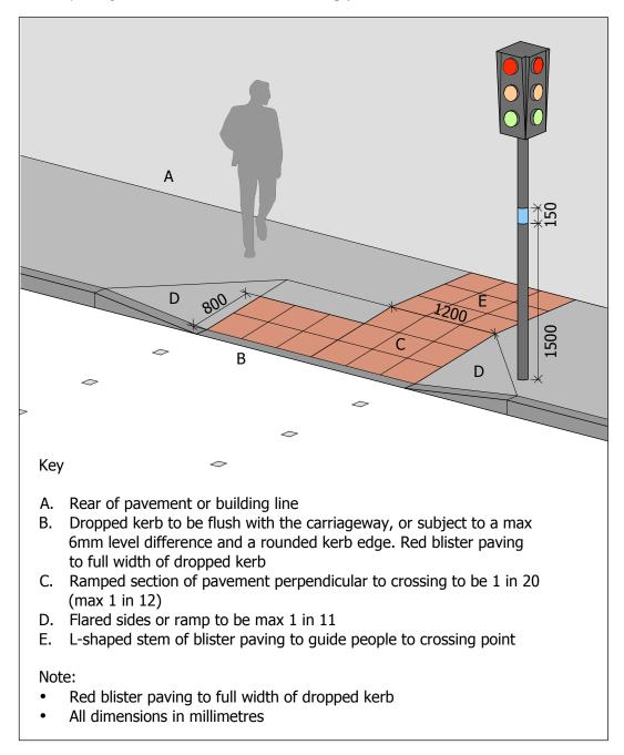
The flared sides of the ramp may have a gradient not exceeding 1 in 11. The ramped section should have a width between 1200mm and 3000mm, dependent on the intensity of use.
