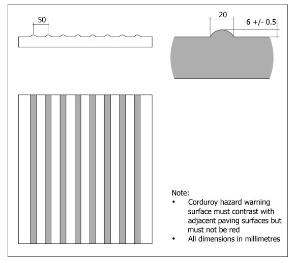
Figure 1.14 Corduroy hazard warning surface.
