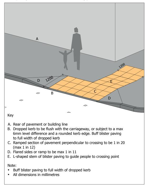
**Figure 1.17b** Crossing point **not** in the direct line of travel. Dropped kerb and buff blister paving surface at **uncontrolled crossing points**.
