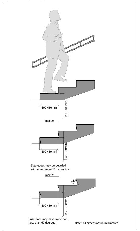
The dimensions of steps should be consistent throughout a flight. The rise of external steps should be in the range 150 to 180mm. The going (depth) should be in the range 300 to 450mm.
