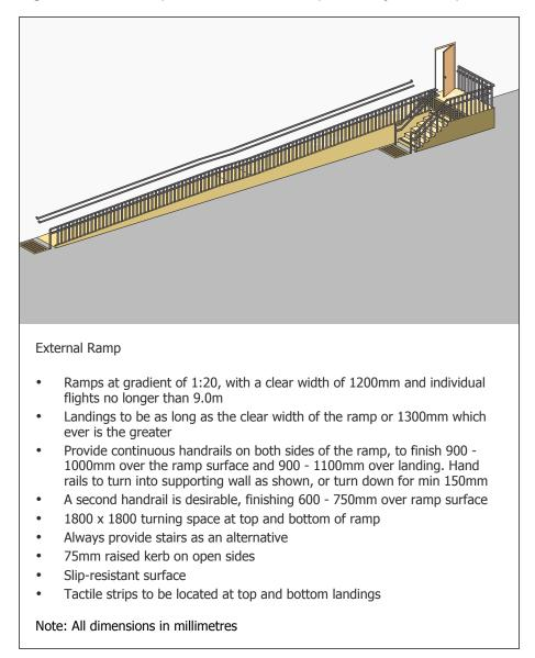
Figure 1.7 An example of an external ramp with adjacent steps.
