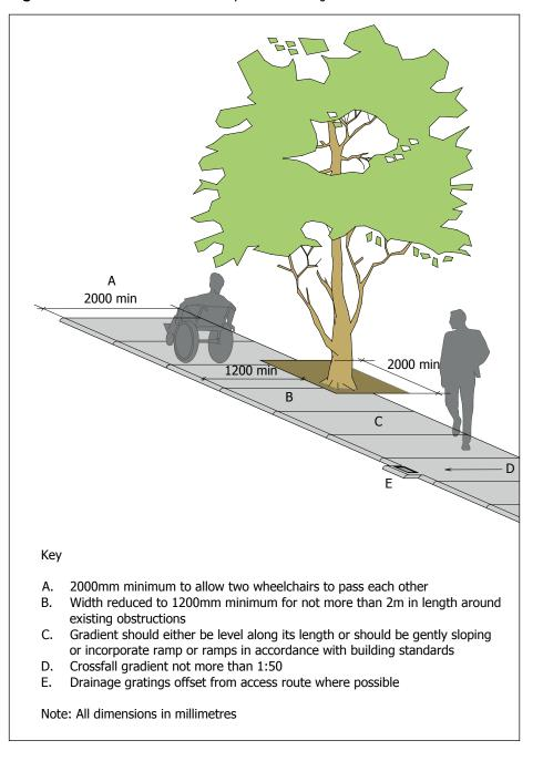
Figure 1.6 Urban environment pavement layout.
