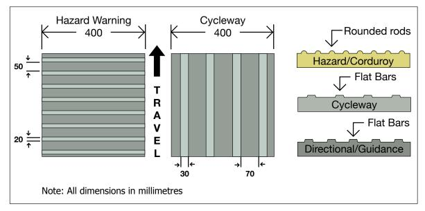
Figure 1.20 Examples of hazard warning and cycleway paving.
