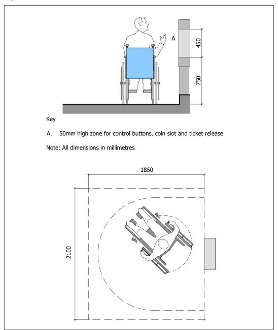
If ticket machines are mounted on a plinth, the edges of the plinth should not project beyond the face of the machine as this can make approach difficult for wheelchair users.
