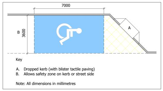
Note: Where designated parallel parking bays are provided in series, or in combination with standard parking bays, an additional 2000mm buffer zone should be provided at the rear of the designated space. The length of the designated parking bay may be reduced to 5800mm long in this instance. (Extract from Department of Transport 'Traffic Signs Manual').
