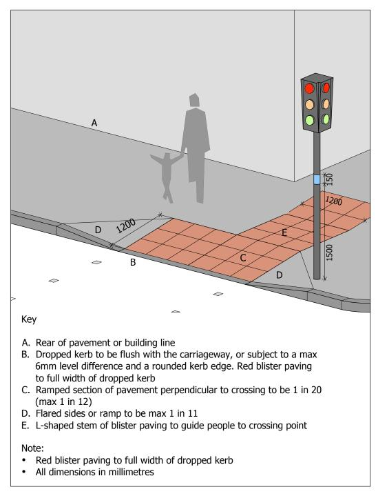
**Figure 1.16b** Crossing point not in the direct line of travel. Dropped kerb and red blister paving surface at **controlled crossing points**.
