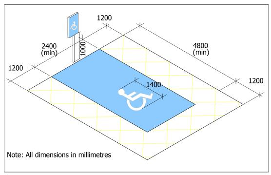
Figure 1.1 Example of perpendicular parking.
