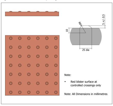
Figure 1.18 Blister tactile paving surface.
