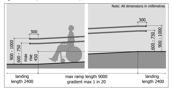
Figure 1.8 Example of an external ramp.
