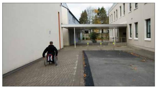
Where the clear width of an access route is less than 2000mm, passing places should be provided. Passing places should be 2000mm wide x 2500mm long, at a reasonable frequency and located within sight of another passing place, subject to a maximum distance of 25m. This will allow groups of people to pass each other, particularly on busy routes. On long routes, level resting places should be provided off the path of travel at intervals of no more than 30 metres.
