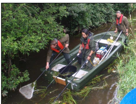
Plate 3.2. Electric-fishing using boat-based electric-fishing equipment
