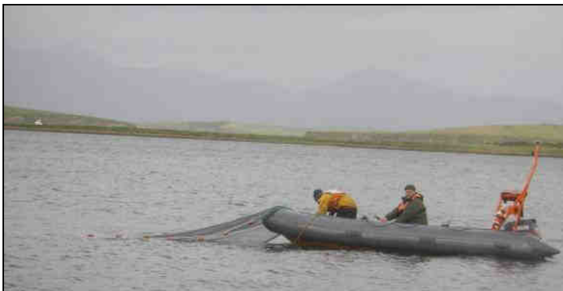
Plate 3.5. Beach seining: deploying the net from a boat
