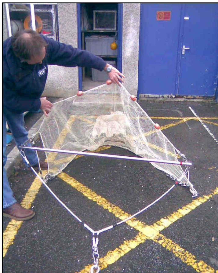
Plate 3.8. Beam trawl used for transitional water surveys
