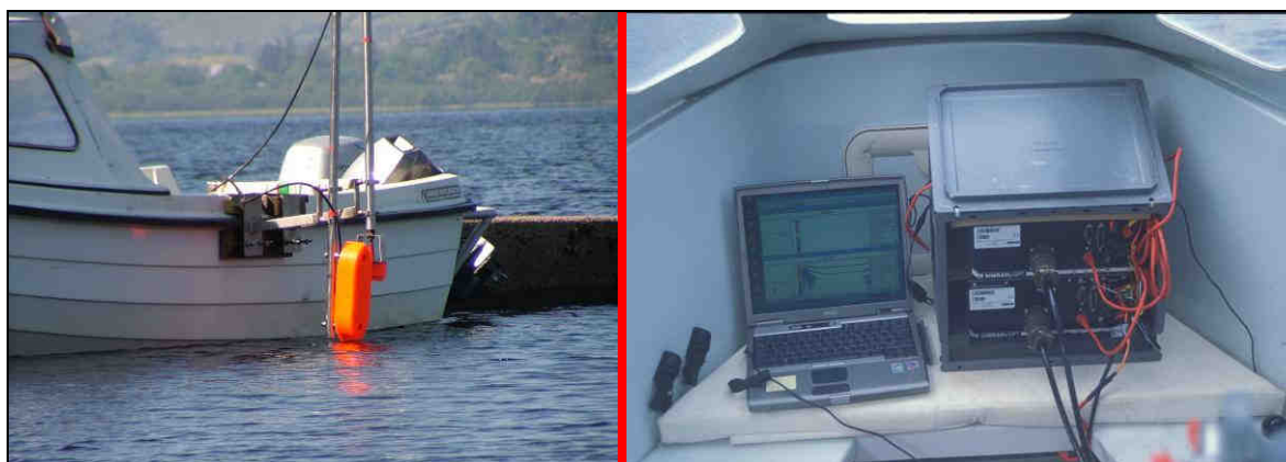
Plate 3.12. Left: Hydroacoustic transducers mounted on a boat (front - horizontally beaming, rear - vertical beaming). Transducers are lifted out of the water for illustrative purposes. Right: Laptop computer controlling the transducers via General Purpose Transceivers (GPT).
