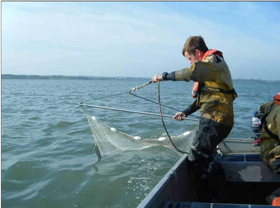
Plate 3.9. Beam trawl used for transitional water surveys
