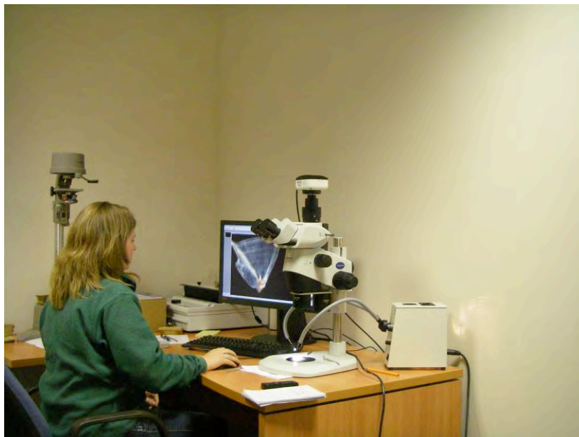
Plate 3.10: Perch aging inter-calibration exercise between an old epidioscope and the new Olympus microscope with image analysis software
