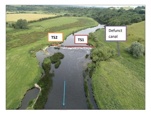
Figure 20. The two transversal sections of Newgrange Weir. Drone imagery taken 15/07/2021.
