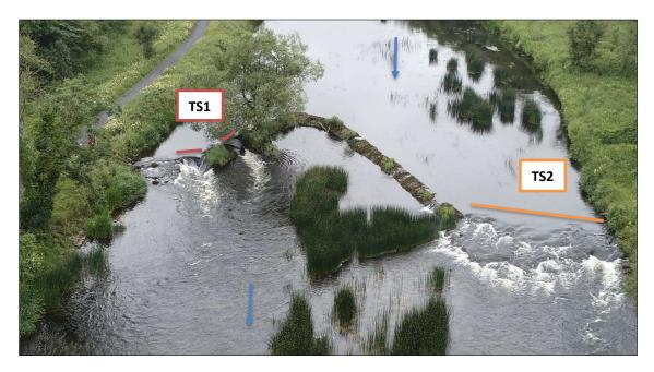
Figure 55. The two transversal sections of Ardmulchan Weir 1. Drone imagery taken 13/07/2021.
