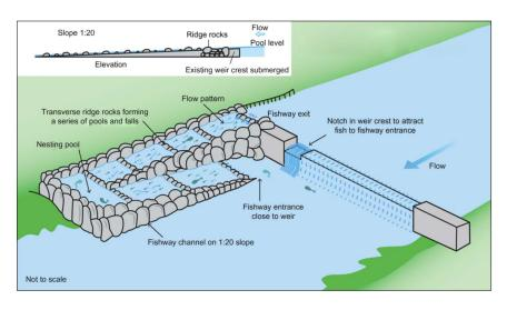
Figure 91. Illustration of partial-width pool and boulder rock-ramp fishway (Thomas, 2017).
