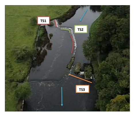
Figure 76. The three transversal sections of Blackcastle Demesne Weir 2. Drone imagery taken 22/09/2020.
