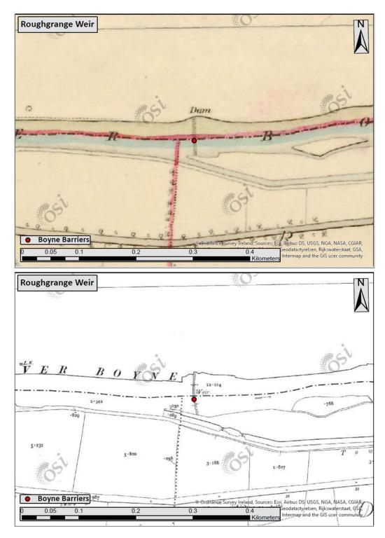
Figure 15. Location of Roughgrange Weir as shown on the historic 6" First Edition OSi map, 1829-1841, (top) and on the Historic 25" OSi map, 1897-1913, (bottom). The structure was originally labelled as a "Dam" but is referred to as a "Weir" in later map editions.
