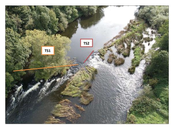
Figure 60. The two transversal sections of Ardmulchan Weir 2. Drone imagery taken 29/09/2020.
