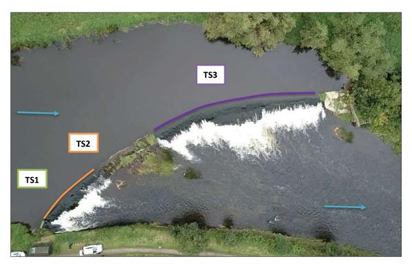
Figure 65. The three transversal sections of Dunmoe Weir. Drone imagery taken 22/09/2020.
