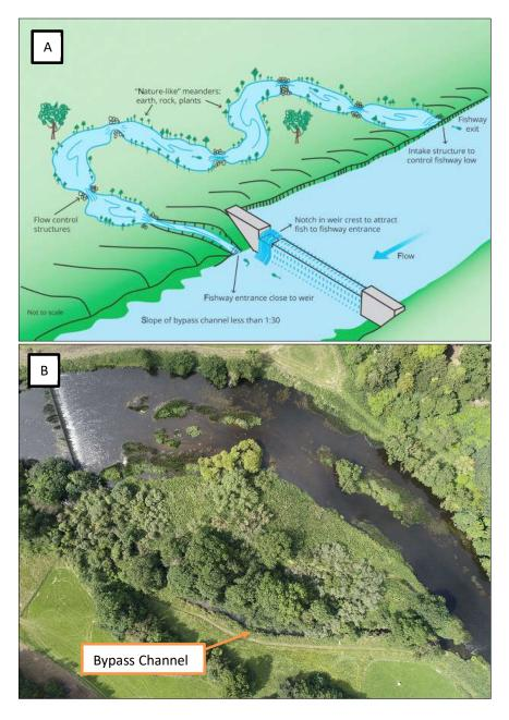
Figure 90. A) Illustration of a bypass channel for promoting the passage of fish and other stream biota (Thomas, 2017). B) Bypass channel on the River Boyne mitigating a weir by Slane Castle. Drone imagery taken 13/07/2021.
